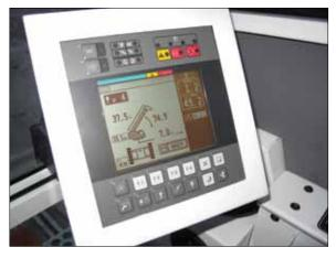
TADANO AML-C rated capacity indicator provides continuous feedback of crane lift position and data.
